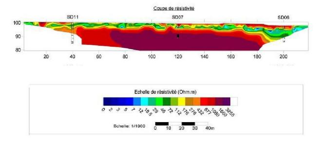
There are inherent limitations to the method and the reversal process: definition decreases with depth. It is important to keep this in mind when comparing resistivity imaging results to geotechnical data. Moreover, a clear boundaries between two materials are not manifest enough on ERT images.
